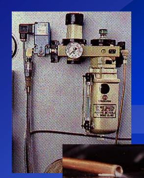
Lubrication system to lubricate the work piece to be beveled
